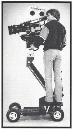
With the boom raised fully the camera lens reaches a height of 67". Camera Risers can be added for additional height.
